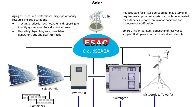
Optimize production operations with supervised control supporting remote access utilizing automatic reconnect/restart process and notification of any underperformance specified to current conditions.
